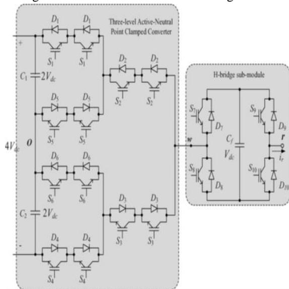
Fig. 1. Circuit configuration of the hybrid Seven-level ANPC-based multilevel converter
