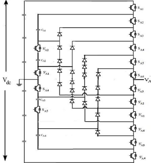
Fig. 2. A phase leg of the proposed 7-level hybrid topology
