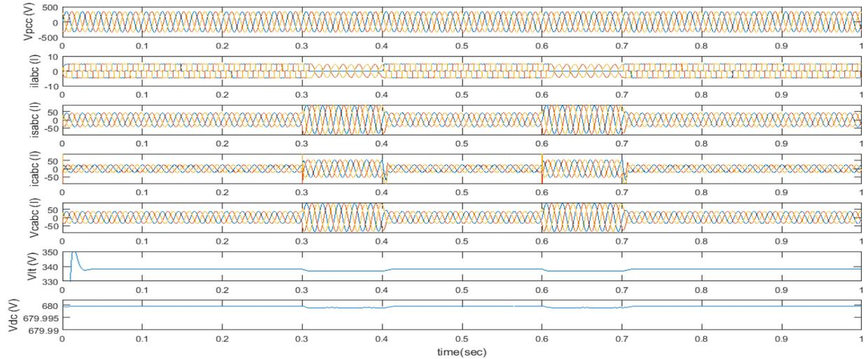
Fig. 5 Analysis of PI-SRF based effective control for DSTATCOM under unbalanced N-L load
