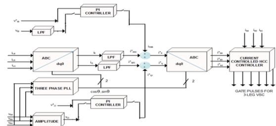
Fig. 3: Control Scheme of PI-SRF algorithm for DSTATCOM.
