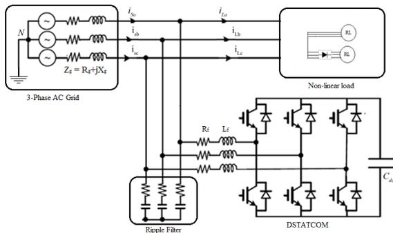
Fig. 2: Circuit structure of DSTATCOM based system.
