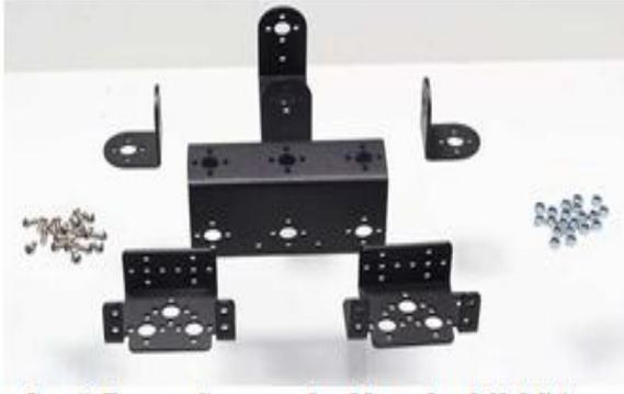
Step 24: Now we will fix the Servo Motor in the two hands. Take 4 x Servo Motors, 16 x M4 Screws and 16 x M4 Nuts.
