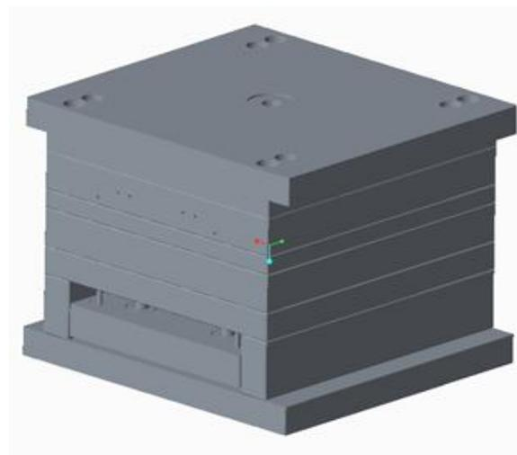
Figure No. 5 Assembly of mould tool.
