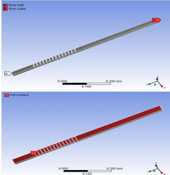
Figure 5 Name selection of corrugated plate heat exchanger
