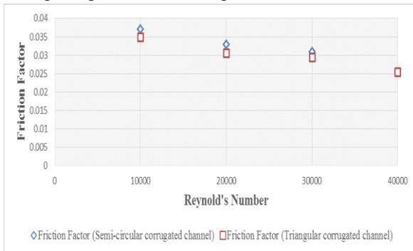
Figure 13 Comparison of Friction Factor at different Reynold's number for Semi-circular and triangular corrugated plate heat exchanger.
