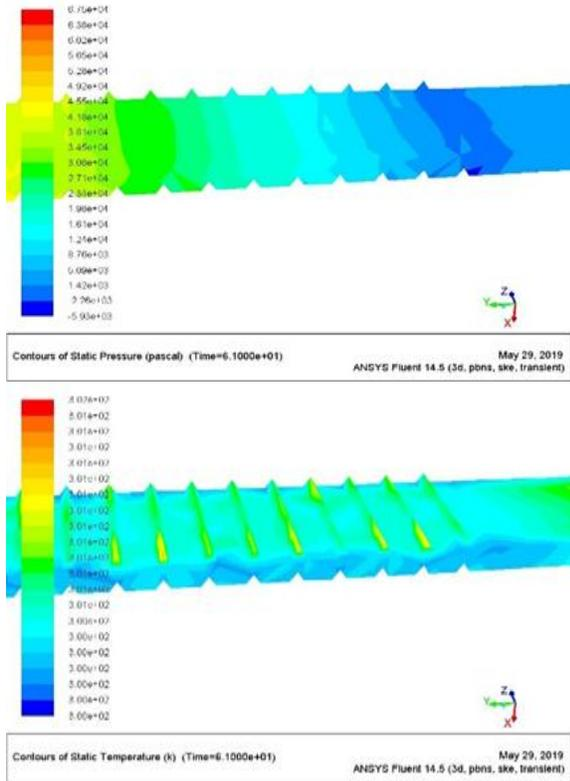
Figure 7 Contours of static pressure and temperature for triangular corrugated at Re=20000
