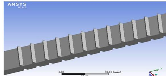
Figure 2 Triangular corrugated channel (test section).
