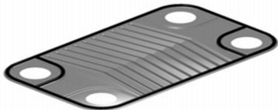
Figure 1: An individual plate for a heat exchanger
