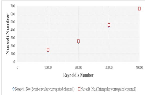
Figure 12 Comparison of Nusselt number at different Reynold's number for Semi-circular and triangular corrugated plate heat exchanger
