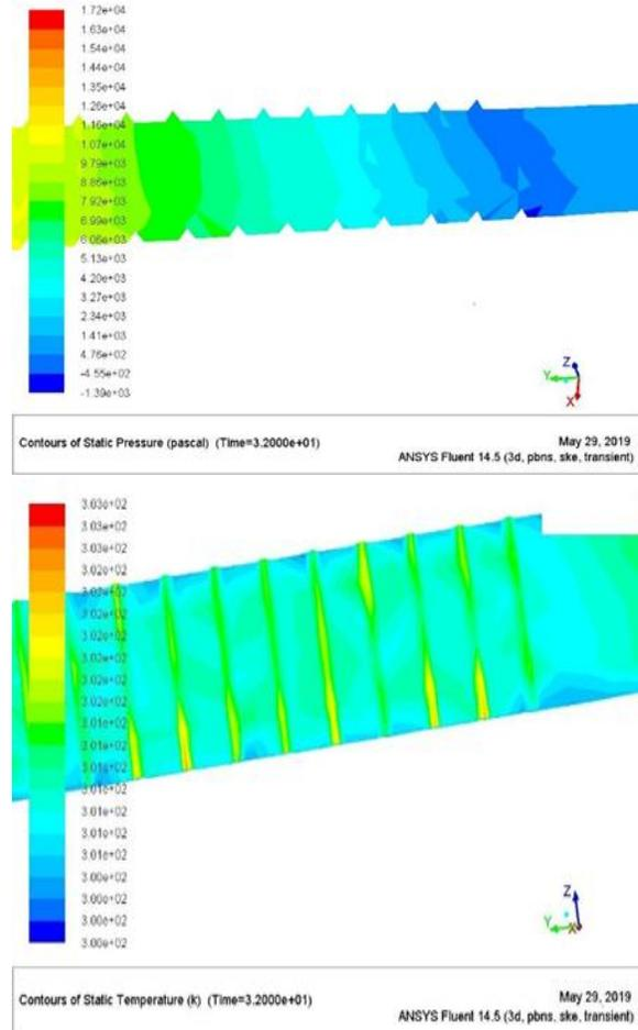
Figure 6 Contours of static pressure and temperature for triangular corrugated at Re=10000
