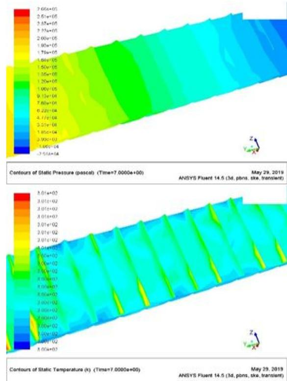
Figure 9 Contours of static pressure and temperature for triangular corrugated at Re=40000
