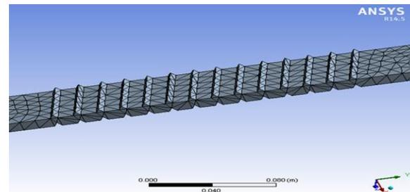
Figure 4 Mesh view of corrugated channel
