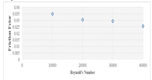
Figure 11 Variation in Friction factor at different Reynold's number.
