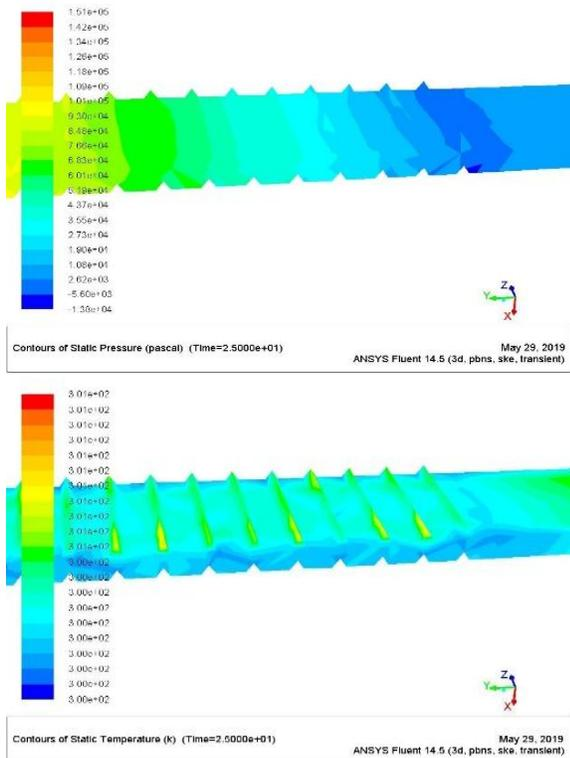
Figure 8 Contours of static pressure and temperature for triangular corrugated at Re=30000
