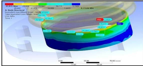
Figure 1.16 Equivalent stress of bellow ring
