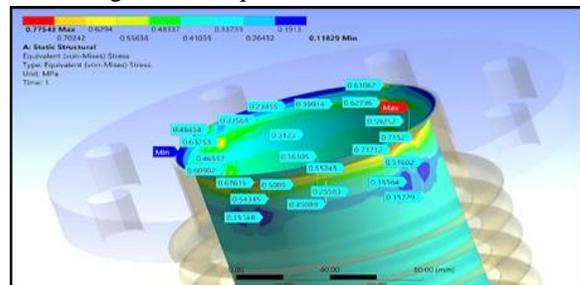
Figure 1.15 Equivalent stress of liner
