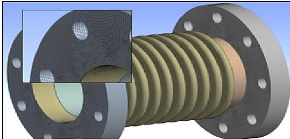
Figure 1.9 ANSYS meshed assembled bellow
