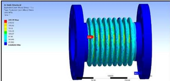
Figure 1.10 Equivalent stress of assembled bellow
