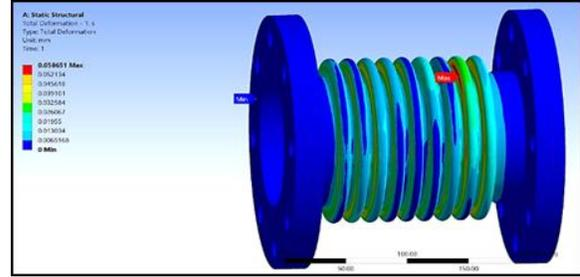
Figure 1.11 Total deformation of assembled bellow
