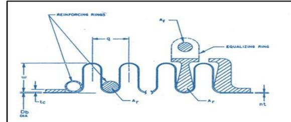
Figure 1.1 Fatigue design of bellow
