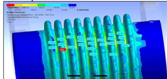
Figure 1.14 Equivalent stress of bellow
