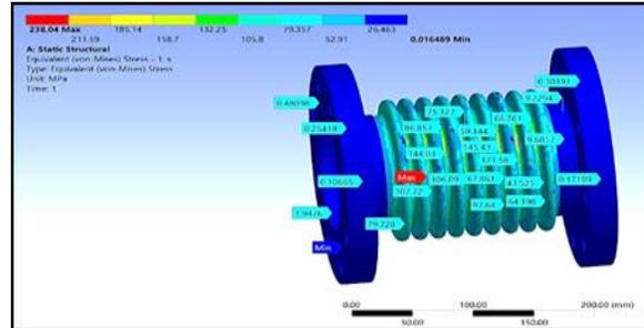
Figure 1.12 Equivalent stress of assembled bellow
