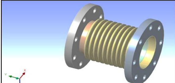
Figure 1.8 ANSYS assembled bellow
