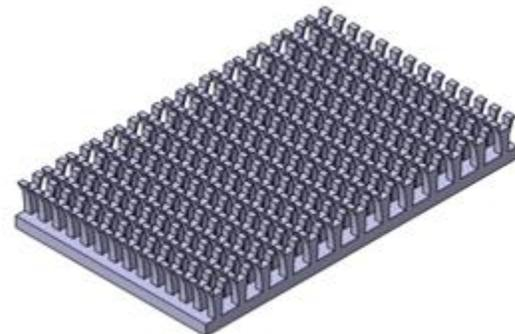
Fig.:4 Fins with Rectangle Notch
