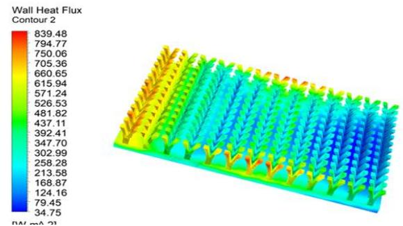
Fig.:11 Heat Flux Changes in Fins with V – Shaped Notch
