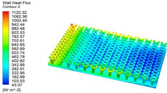
Fig.:12 Heat flux Changes in Fins with Rectangular Notch
