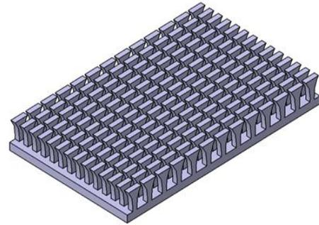
Fig.:1 Fins without any Notch
