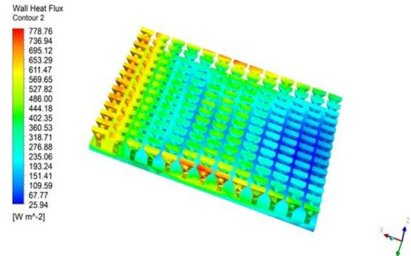
Fig.:10 Heat Flux Changes in Fins with Holes
