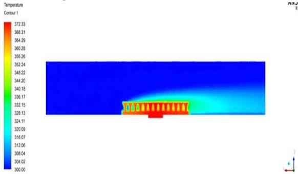
Fig.:5 Heat Flux Change in Normal Fins
