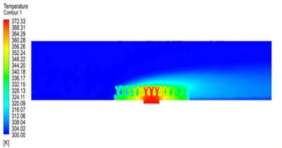
Fig.:7 Temperature Change in Fins with V – Shaped Notch
