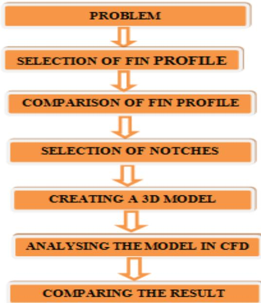
After collecting all the related data's the cooling fins are designed using CREO 2.0. After the model is created the analysis are done by using ANSYS – 14.5 (CFD – Fluent). Then the results of each analysis are compared and then
