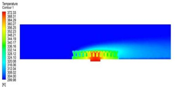
Fig.:8 Temperature Changes in Fins with Rectangular Notch
