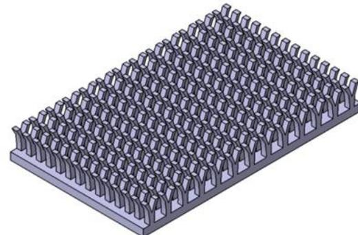
Fig.:3 Fins with V – Shaped Notch
