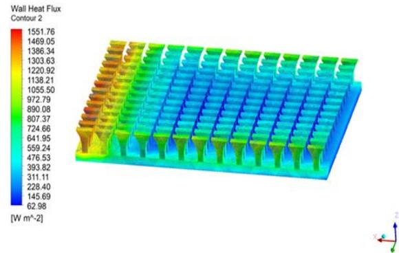
Fig.:9 Heat Flux Changes in Normal Fins
