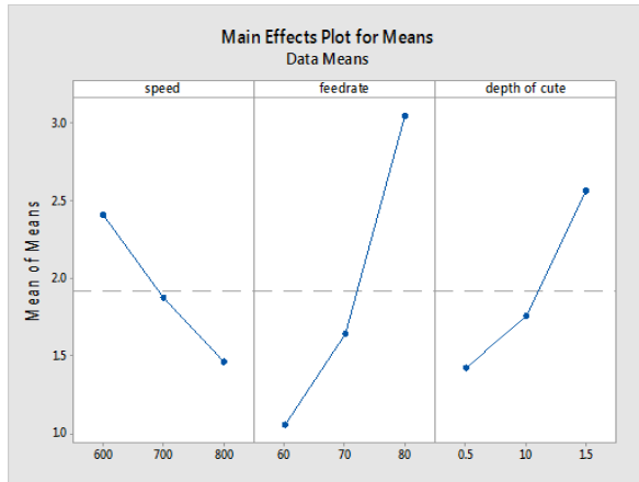
Fig: 5.2 effects of speed, feed rate, depth of cut on milling
