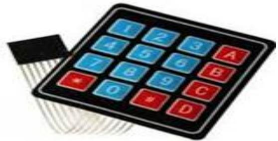
Typically, one port pin is required to read a digital input into the controller. When there are a lot of digital inputs that have to be read, it is not feasible to allocate one pin for each of them. This is when a matrix keypad arrangement is used to reduce the pin count. Therefore, the number of pins that are required to interface a given number of inputs decreases with increase in the order of the matrix.
