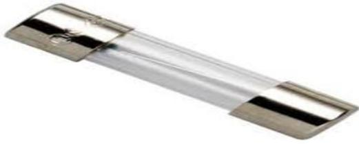
A fuse is an electrical safety device that operates to overcurrent protection of an electrical circuit. Its essential component is a metal wire or strip that melts when too much current flows through it, thereby interrupting the current. It is sacrificial device. Once a fuse has operated it is an open circuit, and it must be replaced or rewired, depending on type. Here we are using 250V fuse that will interrupt a 5A current after 100sec
