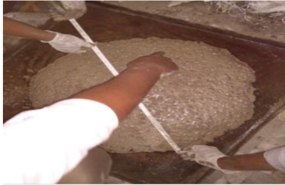
Slump flow of self compacted concrete
