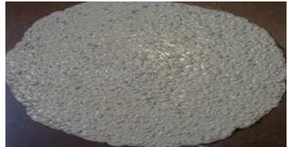
Fig.: Self compacting concrete
