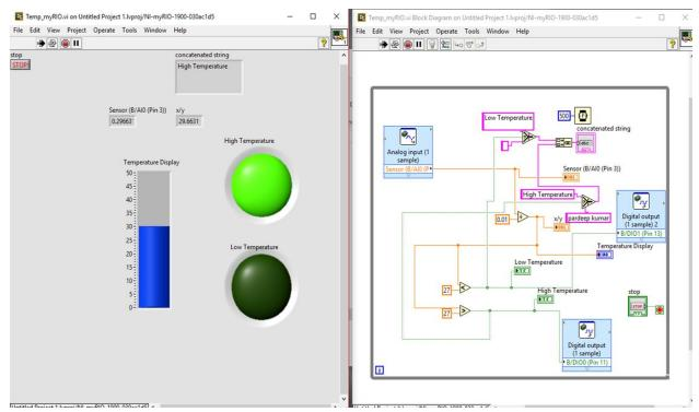
when we touch LM35 sensor than the temperature is increase more than 28 degree C RED led ON show in
