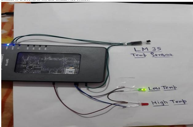
LM35 there have no heat nearby sensor than temperature is less than 28 degree C GREEN Led ON
