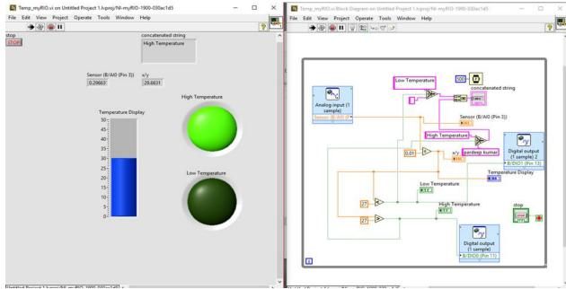
myRIO hardware system connect 2 LED, one is GREEN, second is RED with attach LM35 temperature sensor. In this circuit Green LED –ve Pin connect to B/DIO1(Pin 13) and GREEN led connect
