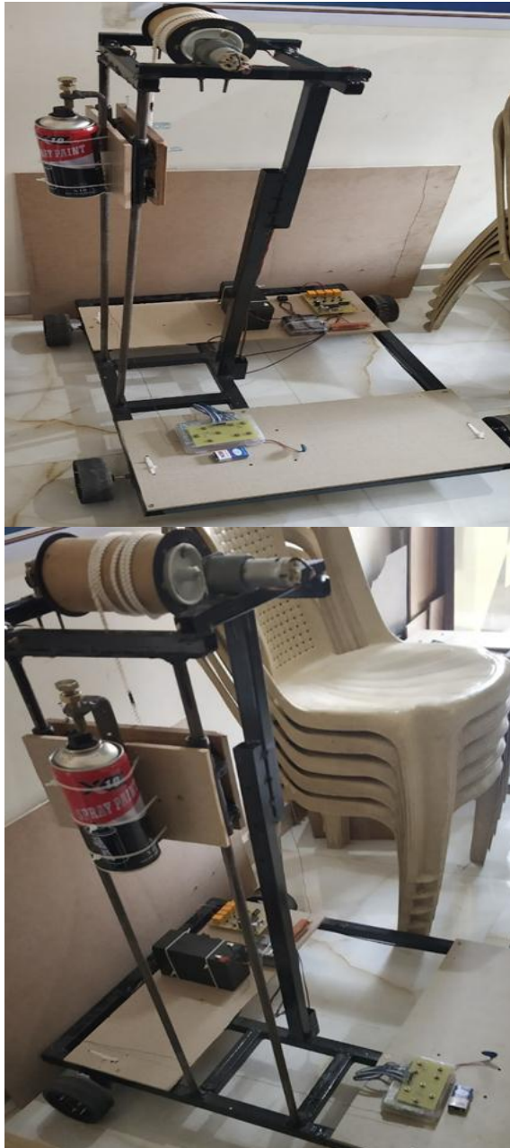
Fig. No. 5.1 Actual Model of Man Free Wall Painting Robot
