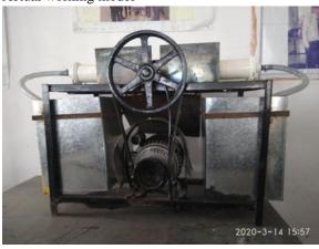
C. Specifications: 1. Motor Maximum Power : 0.5HP Maximum Voltage: 220 V AC Maximum Speed : 1440 RPM Current: 3.5 amps
