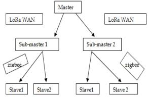
Figure 4 Master-slave network architecture
