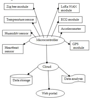
Figure 5 block diagram implementation of the prototype
