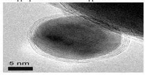
Colloid formation for metallic particles is also much more challenging. Cobalt nanoparticle with graphene shell. Cobalt nanoparticle with graphene shell (note: The individual graphene layers are visible)[28]
