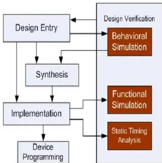
Fig 1: Design Flow of FPGA
