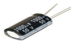
A capacitor is a device that stores electrical energy in an electric field. It is a passive electronic component with two terminals. The effect of a capacitor is known as capacitance. No current actually flows through the dielectric. However, there is a flow of charge through the source circuit.
