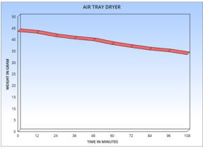
Fig. 1 Air Tray Dryer Graphical Representation
