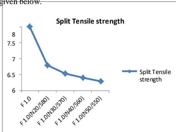
Fig -3: Split Tensile Strength of SCC
