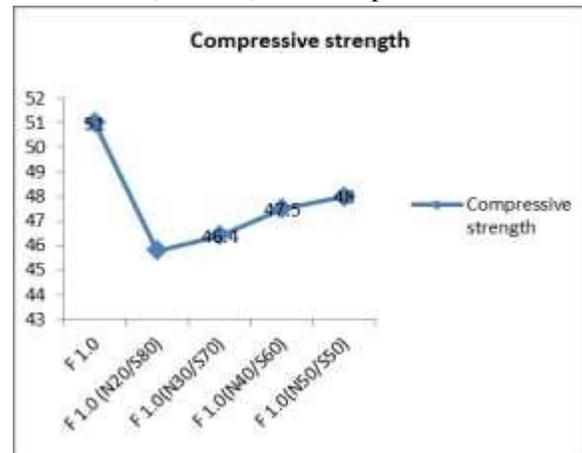
Fig -1: Compressive Strength of SCC
