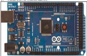
The Arduino Mega 2560 is a microcontroller board based on the ATmega2560 (datasheet). It has 54 digital input/output pins (of which 14 can be used as PWM outputs), 16 analogy inputs, 4 UARTs (hardware serial ports), a 16 MHz crystal oscillator, a USB connection, a power jack, an ICSP header, and a reset button. It contains everything needed to support the microcontroller; simply connect it to a computer with a USB cable or power it with an AC-to-DC adapter or battery to get started. The Mega is
