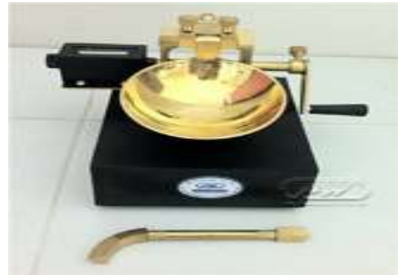
Fig 4.4.1: .Casagrande's Liquid Limit Device
