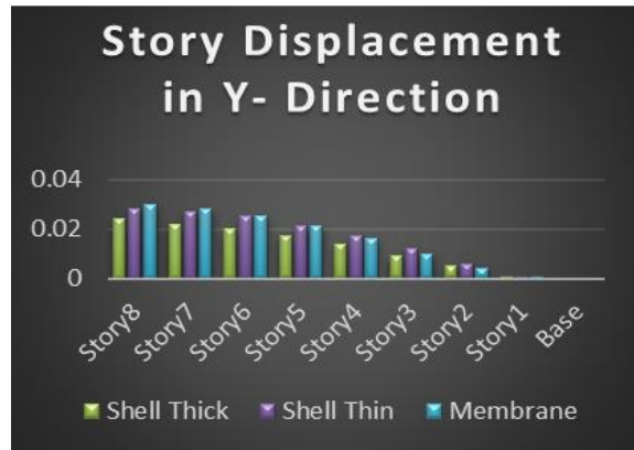
Figure 4.2 comparisons of story displacement in y direction
