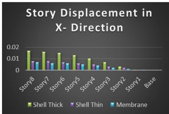
Figure 4.1 comparisons of story displacement in x direction
