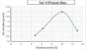
Figure 3.4 Soil + 0.8% plastic fiber
