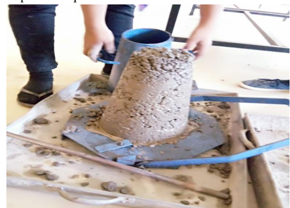
Fig. Slump cone testing
