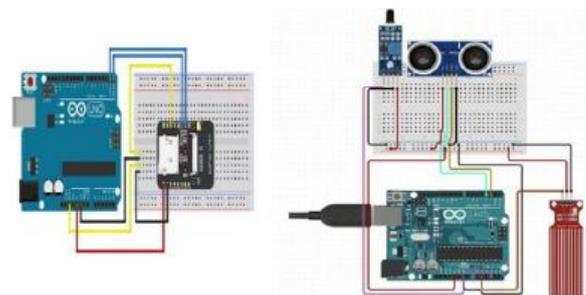
Fig. 1: Connection diagram of Smart Stick for Blind
