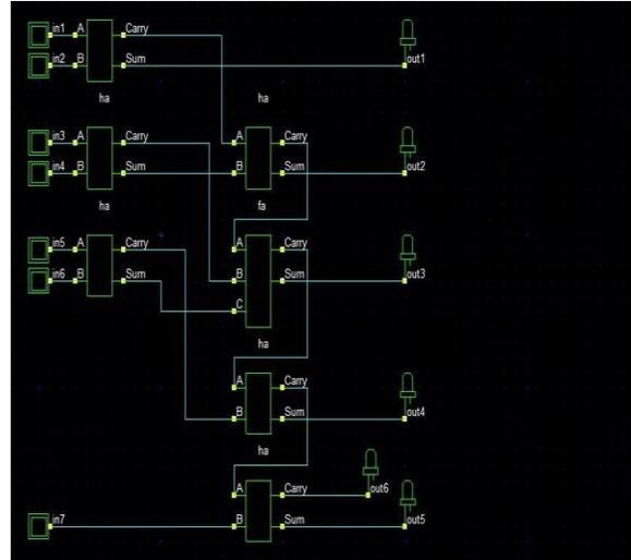
Fig 4.3: Schematic Design of Carry Save Adder 2
