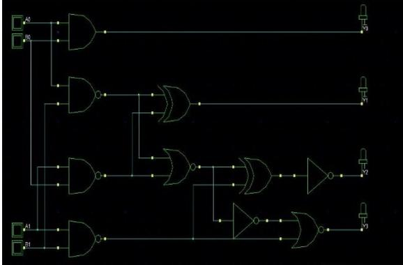
Fig 4.1: Schematic Designing of 2 – Bit Multiplier. The 4 × 4 multiplication is done considering the grouping 2 bits together each of the 4 – Bit input.
