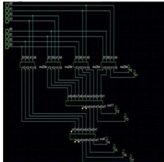
Fig: Schematic of 4 – Bit Vedic Multiplier
