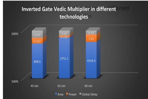
From the figure we can observe the area, power, delay in different Gpdk TSMC technologies those are 45, 65, 90 nm Gpdk technologies. As per our observation compared to 45 nm with 65 nm technology 45 nm technology is better because of while comparing their parameters like power, delay and area. 65 nm technology consumes more. And compared with 65 nm with 90 nm technology 65 nm technology is better, while comparing 45, 65, 90 nm Gpdk technologies 45 nm technology best one.
