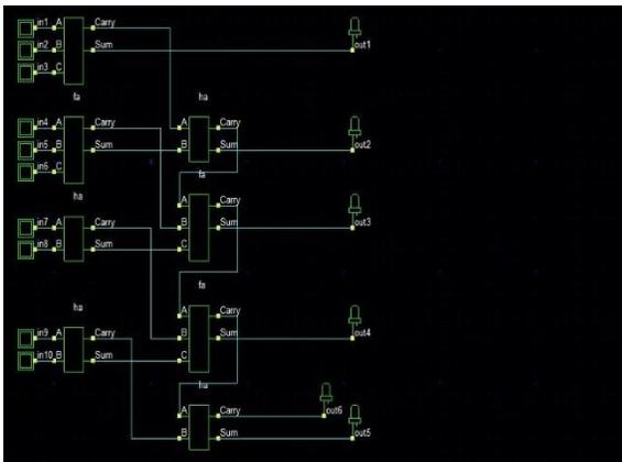
Fig 4.2 : Schematic Design of Carry Save Adder 1
