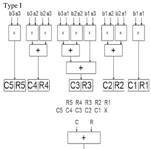
In this architecture 9 multipliers each of 4 bits, 4 adders of 8bits and 9 bits are used respectively
