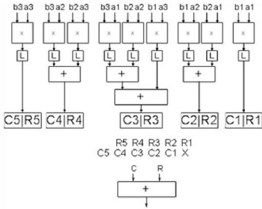
In this architecture pipeline approach has been implemented and latches have been used. Latches are used to stabilize the initial state.
