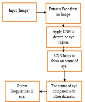
Figure 6, the workflow of the Algorithm-I Procedure With using the MTCNN (Multi-Tasking Convolution Neural Network) Algorithm, the face region of a model has been determined, and in the second step, the facial landmarks of a model are marked, which can be seen in figure 7
