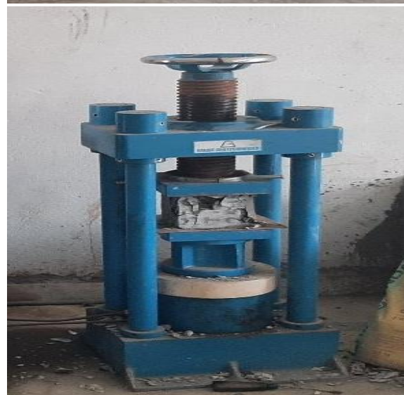
Figure 4: Arrangement & Failure of Specimen
