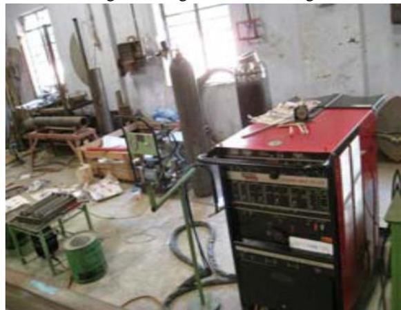
Figure 2 Lincoln Electrical square wave TIG 355 GTAW machine
