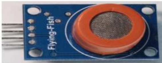
Fig 4. Alcohol sensor that acts as a breath analyser
