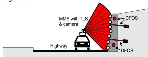
Figure 12. Example of a modern monitoring setup of an anchored retaining wall
