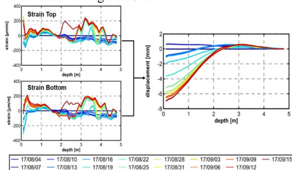
Figure 11. Strain profiles along the top and bottom of nail #1 and derived displacement curve
