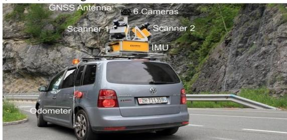
Figure 3. Mobile mapping system mounted on a car. The used MMS consists of a geodetic GNSS antenna with a receiver, an inertial measurement unit (IMU), two laser scanners, six cameras and an odometer. The entire measurement platform is mounted on a standard car. The position of the platform is calculated using differential GNSS and supported by the IMU and odometer data. The orientation is mainly determined with the IMU. The two laser scanners work in profile
