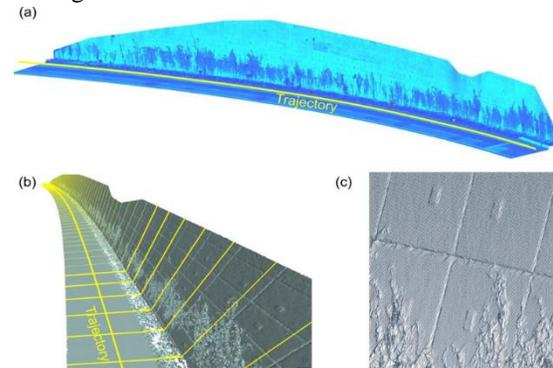
Figure 4. Point cloud (a) and TIN model (b) of the highway surface and retaining wall. The car trajectory and vertical profiles every 5 m are indicated as yellow lines. Detailed profiles (c) every 5 cm along the trajectory are used for further processing.
