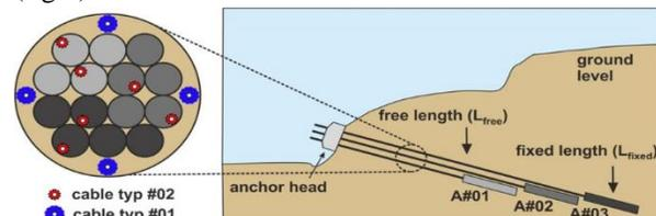
Figure 8. Schematic representation of single borehole multiple anchors with two sensing fibres along the
