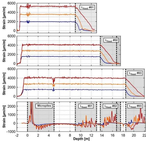
Figure 9. Measured strain profiles at load steps of 900, 1500 and 2100 kN along the anchor tendons of the short (#01), middle (#02) and long (#03) SBMA anchor and the grout material
