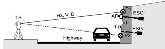
Figure 1. Conventional monitoring setup of an anchored retaining wall
