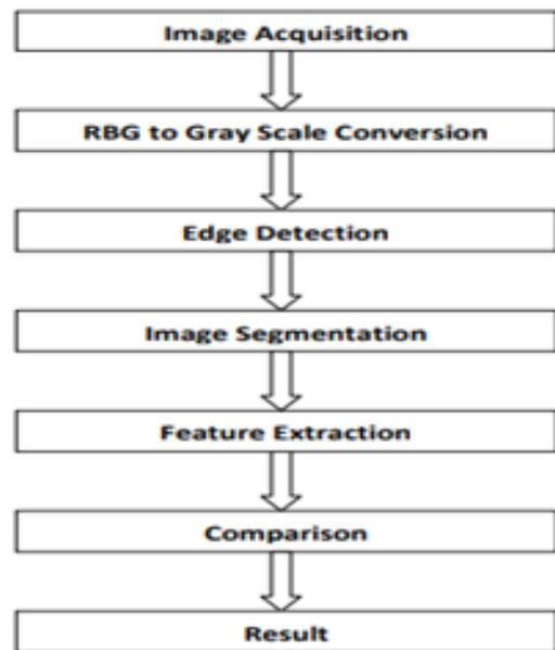
Fig: Block diagram of Indian Currency Detection System
