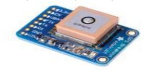
The idea of tracking something is cool enough but doing so without a telephone or an internet connection is much cooler. The whole GPS system depends on 24 (minimum) satellites orbiting the earth. Each satellite continually broadcast their current time and position. Generally, a GPS receiver requires a connection to at least four of these satellites to acquire data to compute for position. The receiver also computes for the clock difference between it and the satellite.
