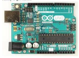
Features of Arduino UNO It contains ATMEGA328P Micro Controller It is a 8-bit microcontroller.
