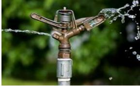
Sprinklers can be used for residential, industrial, and agricultural usage. It gets sprinkled on the crop. In sprinkler or overhead irrigation, water is piped to one more central locations within the field and distributed by overhead high pressure sprinklers or guns.
