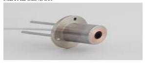
When a metal object enters this field, eddy currents are induced into the object. As the metal moves closer to the sensor, these eddy currents increase and result in an absorption of energy from the coil which dampens the oscillator amplitude until it finally stops.
