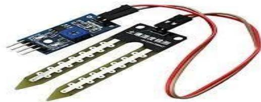
The soil sensor, which stipulates the wetness of the soil, measures the volumetric contents of water inside the earth and gives us the moisture level as output. The sensor averages the water content over the entire length of the soil environment, wet or dry and the propelled yield. The sensors can measure temperature
