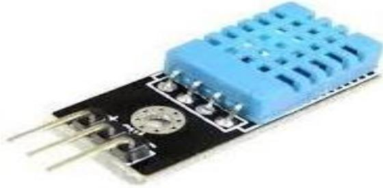
The humidity sensing device DHT11 is a moisture holding substrate with the electrodes applied to the surface. The change in resistance between the two electrodes is proportional to the relative humidity. Humidity sensors work by detecting changes that alter electrical currents or temperature in the air.[2]
