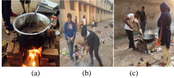
Fig.4: (a) Heating the sand, (b) Adding LDPE over heated sand, (c) Mixing the batch
