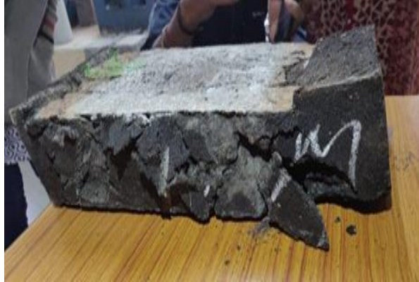
Fig.8: Crushed paver block sample of PB2 after CTM testing
