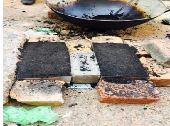
Fig.7: Set paver block just before demoulding
