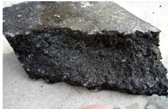
Fig.12: Breaking of PB4 batch sample when dropped from a height of 10m
