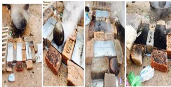
Fig.5: Transferring the mixture of sand and plastic to the mould
