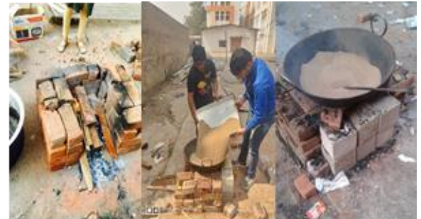
Fig.3: (a) Setup, (b) Adding the filtere sand to the mixing container, (c) Heating it to180oC
