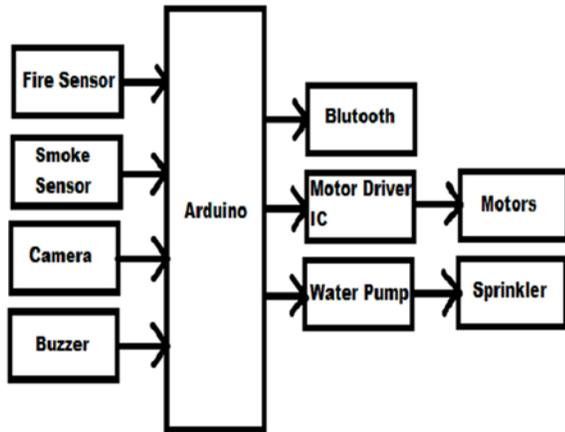
Figure 1:Block Diagram of Fire Extinguisher Robot
