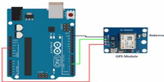
fig 7. GPS Interfacing
