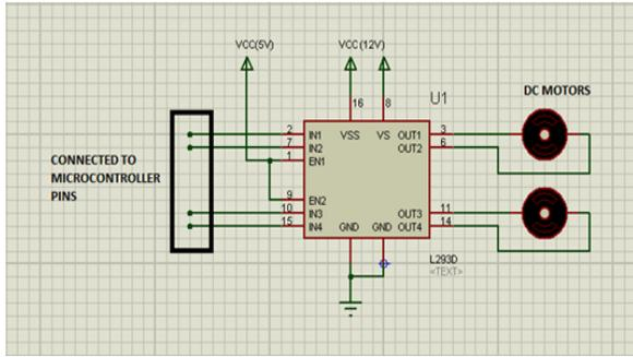
fig 5. Motor Interfacing
