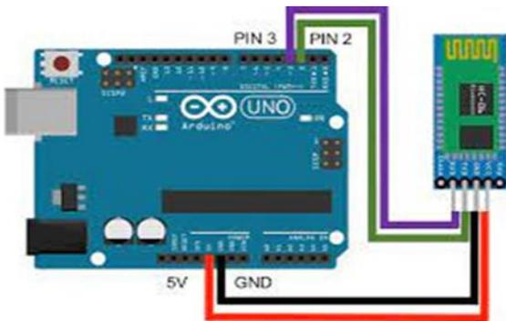
fig 6. Bluetooth Interfacing
