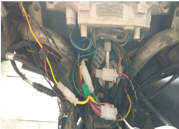
Next, we have to connect the battery wire through the controller, we have to use MCB for the safety purpose of the positive terminal for MCB. We will use the compactable socket for the battery to connect a wire
