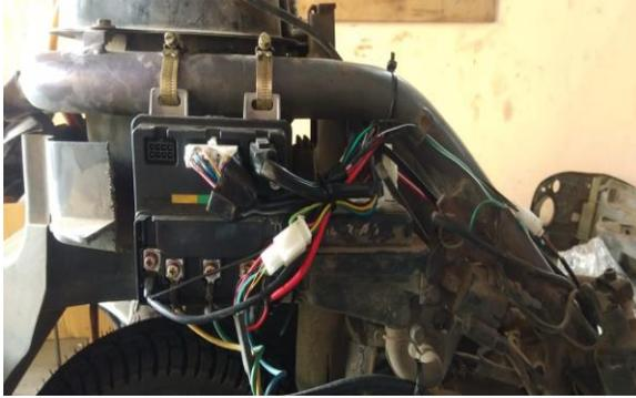
Next, we have to fix dc-dc converter, starter button, battery level indicator. From the controller three core wire was passed to the front panel, we will take 12v relay from the relay we have to connect led switch and dc-dc converter and scooter battery. With the help of a multimeter, we have to find by which wire we are getting 12v we have to connect one wire from the battery to the led switch. So, the wiring part will complete between all components.
