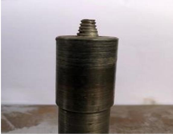
Fig. 3. Conical threaded tool pin profile used for experimental work
