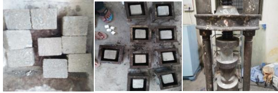
Preparation of specimens and testing for compressive strength
