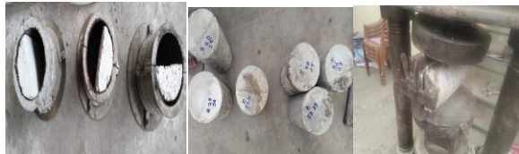
Preparation of specimens and testing for split tensile strength
