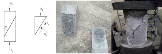
Preparation of specimens and testing for slant shear strength
