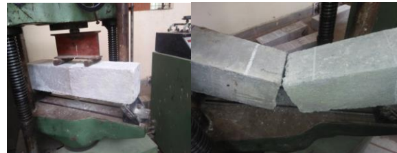
Testing specimens for flexural strength
