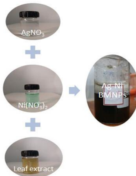
Figure (1): Synthesis of Ag-Ni HNPs from precursor solutions
