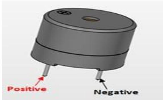
Fig 4: Piezo Buzzer
