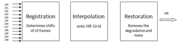
Figure 1: Common Super Resolution Flow Diagram Detailed study of existing techniques in Super-Resolution was done with the help of different literatures available in journals and books. A Proliferation of literature is available in Super-resolution. Here highlight some of the key contributions. Super-resolution (SR) can be achieved using a single image or multiple images (image sets). In single image the input is single LR image. But in the case of multiple we take the different images of same scene it will give different looks of same scene. Based on the taxonomy of super-resolution technique based on the transformation domain super-resolution techniques are classified as two 1)spatial domain and 2)frequency domain. In spatial domain it is the normal image space. We perform operations directly on pixels. In frequency domain apply transforms (Fourier transform) convert it as frequency components and perform mathematical operations on this frequency components and again transform it into spatial domain for display purpose. Glasner et. al [20] combined the above two methods so as to obtain super - resolution
