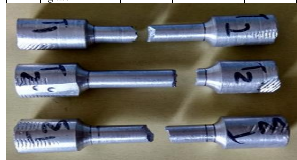
Fig 4.1 Tensile test specimen
