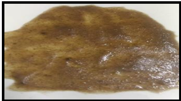
Fig: 5 Bioplastic sheet after 4 days from the formation date
