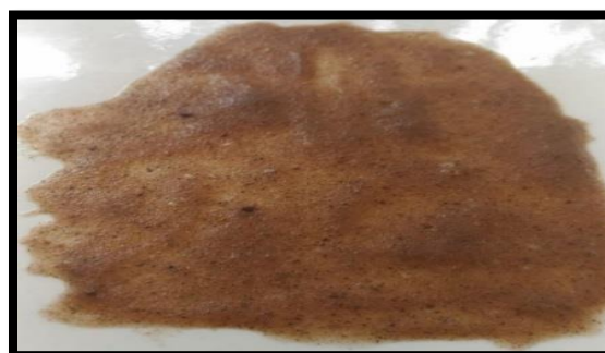
Fig: 4: Bioplastic sheet prepared from jack fruit seed nanopowder
