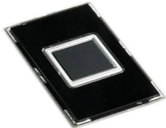
Fig semiconductor finger print module
