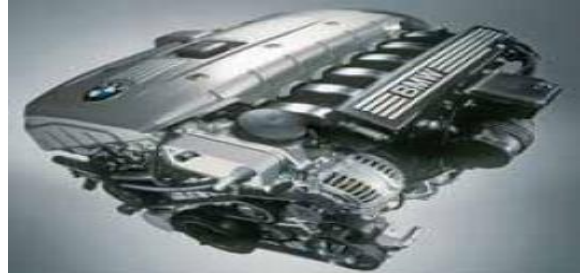
BMW's 6-cylinder R6 power plant uses a magnesium alloy AMC-SC1-fabricated cylinder block
