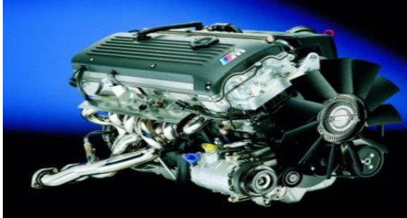
BMW's S54 inline-6 engine, which uses a gray cast iron engine block
