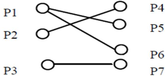
Fig. 6. Tasks allocated to processors, the diagram shows the tasks namely task1, task2, task3 and task4 are allocated to the processors (P1, P5); (P1, P6); (P2, P4) and (P3, P7) respectively
