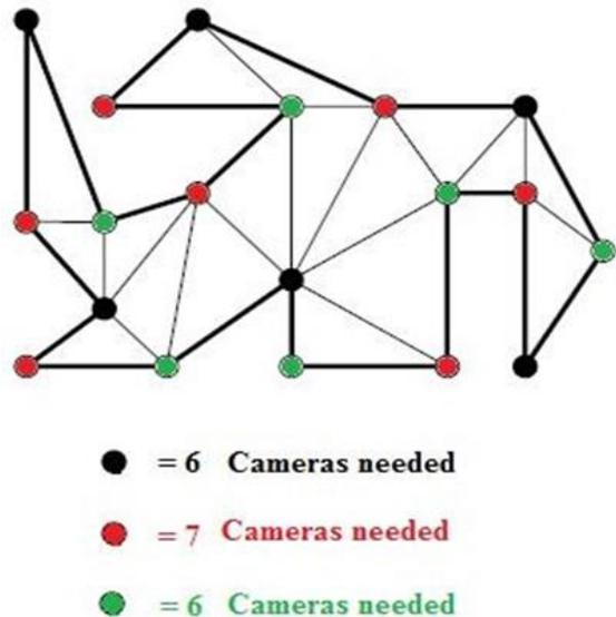
Fig 4. A 3-Coloring of the Triangulated Polygon in Fig 3, take the smallest color class to place the cameras. Here, we can choose black or green color class to place the cameras.
