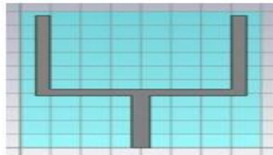
Fig 5: Radiator of proposed antenna
