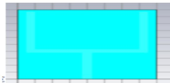
Fig 7: Teslin substrate of proposed antenna
